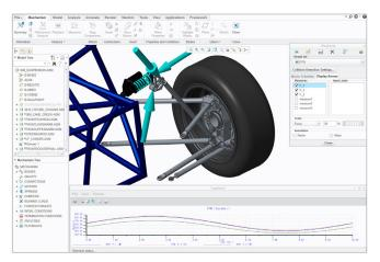
Mechanism Design lets you create mechanical connections and simulate motion on kinetic assemblies.
